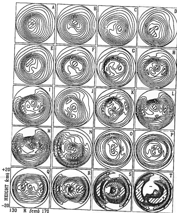
Fig.4. T-10 tokamak. The result of the tomographic reconstruction of the SXR profiles for three angles of registration. The successive instance during the disruption development begins at the top left and goes in alphabet order. The time resolution is 10mks. The time between pictures is 60mks.
